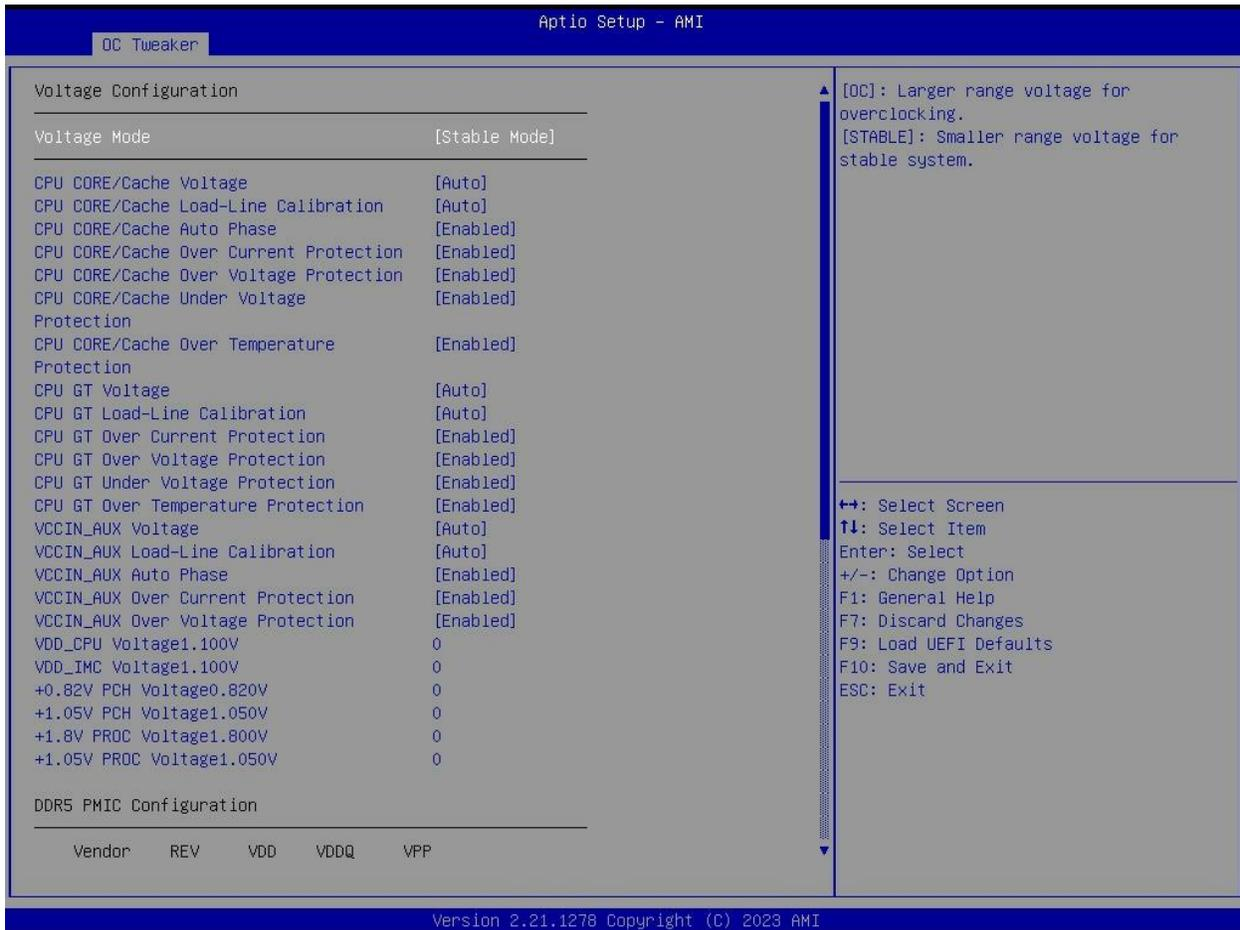
**IMPORTANT NOTE:** Modification of Voltage settings should only be modified and configured by experts. Only the default (Auto) settings are tested and validated by OnLogic. Improper configuration may impact system functionality and/or stability.
