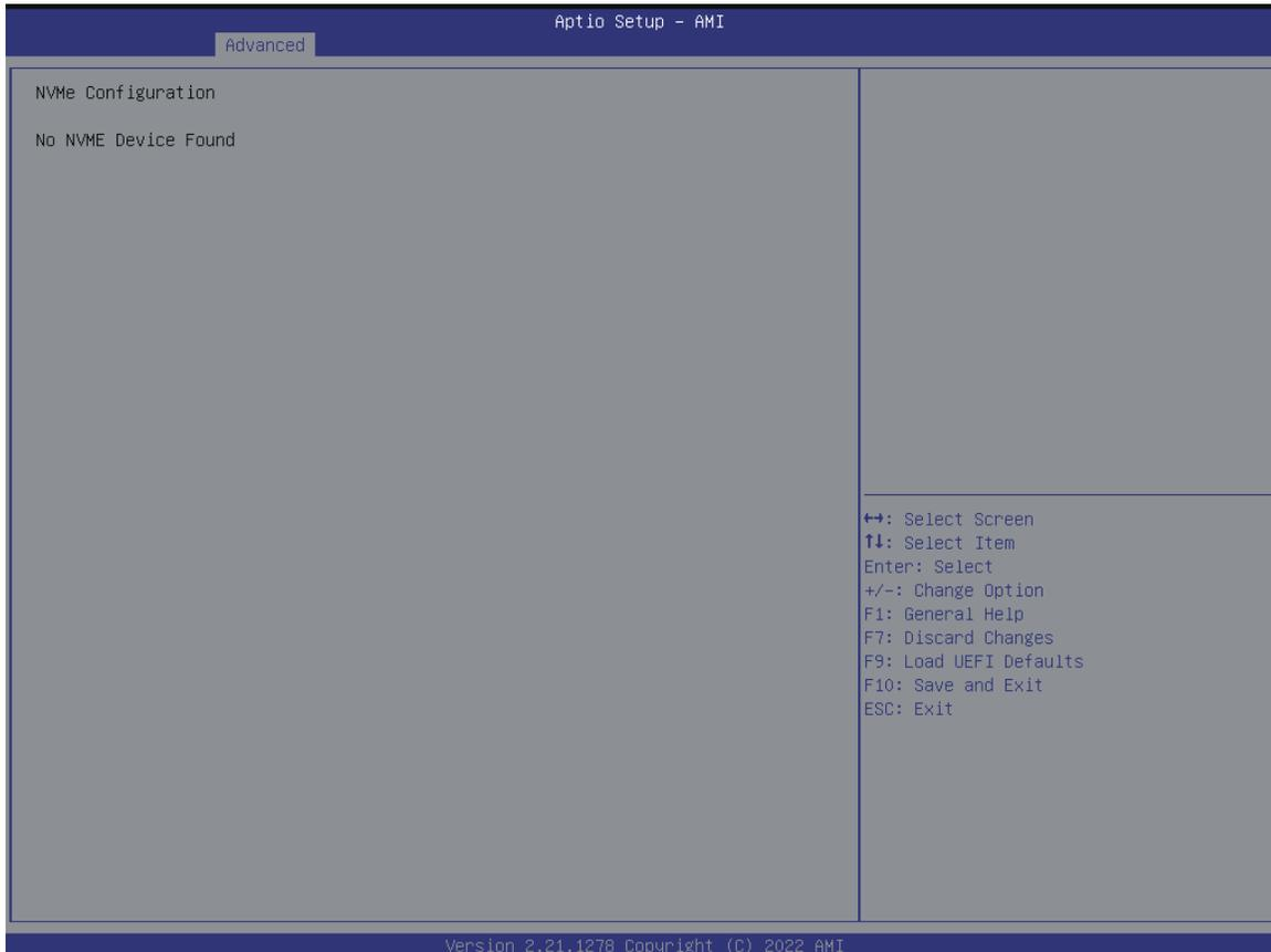
The NVMe Configuration screen displays the NVMe controller and Drive information.
