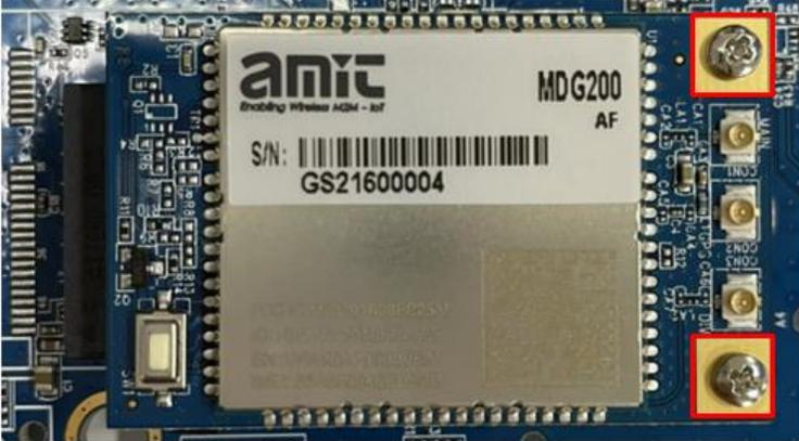
Step 4: Connecting antenna cables accordingly.
