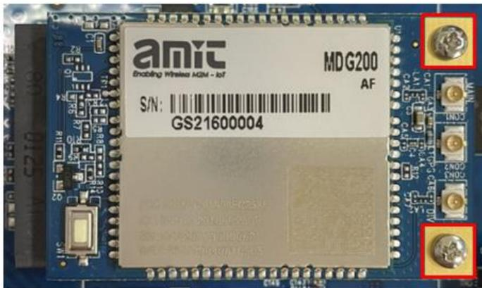
Step 4: Connecting antenna cables accordingly.
