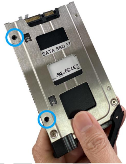
Secure disk with screws
