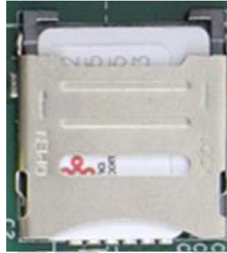
Close and slide to lock SIM in place
