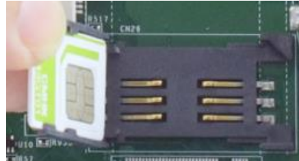
Insert mini-SIM card with pins facing up
