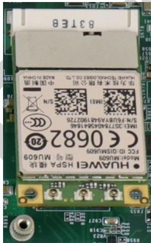
Insert on 45 degree angle
