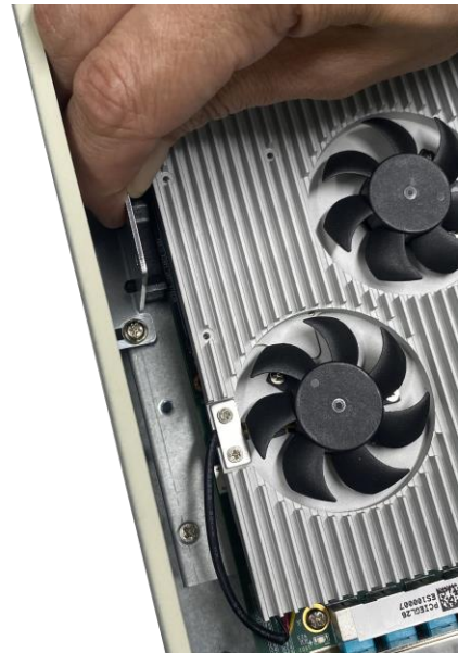
Secure the L-shaped bracket
