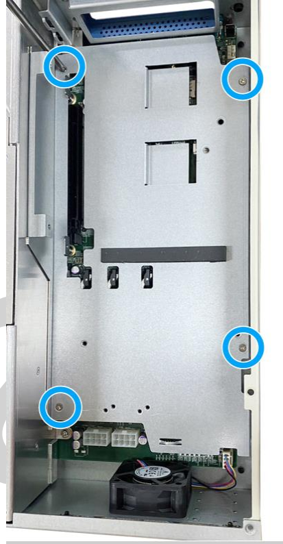
Place and secure the internal platform
